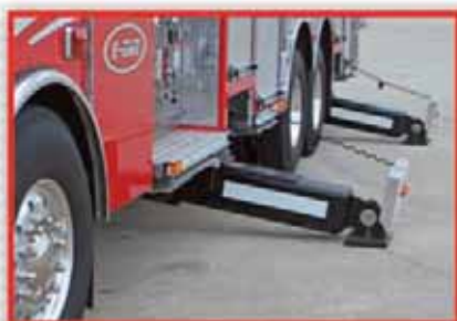
E-ONE EXCLUSIVE CRISSCROSS, UNDER-SLUNG JACK SYSTEM DEPLOYS IN LESS THAN 40 SECONDS.
