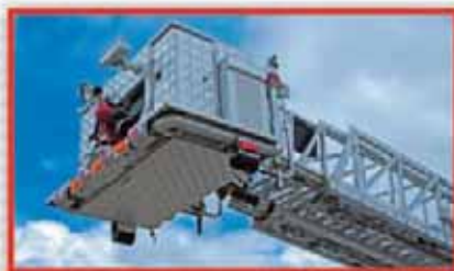
PLATFORM WITH EXTERIOR CATWALK ALLOWS FOR SAFE RESCUE OPERATIONS WITH A CAPACITY FOR THREE FIREFIGHTERS PLUS EQUIPMENT.
