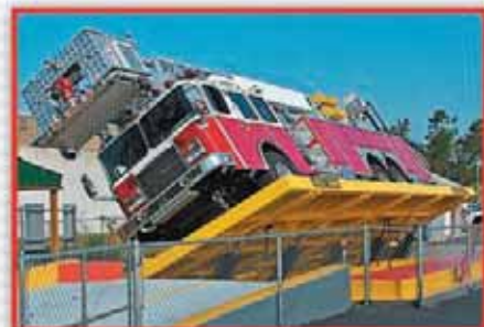
INVESTING IN FIREFIGHTER SAFETY IS OUR PRIMARY CONCERN. THIS TILT TABLE WAS A $500,000 ACQUISITION AND CAN LIFT UP TO 150,000 LBS.
