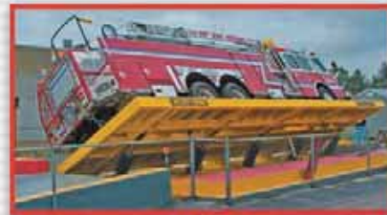
INVESTING IN FIREFIGHTER SAFETY IS OUR PRIMARY CONCERN. THIS TILT TABLE WAS A $500,000 ACQUISITION AND CAN LIFT UP TO 150,000 LBS.
