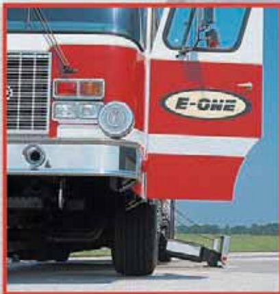
With enough room to open the doors (12 ft. spread), the pin-free jack system is ready to deploy.
