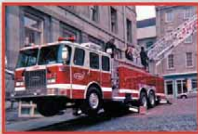
The Exclusive E-ONE under-slung jack system allows easy set-up on hilly terrain.
