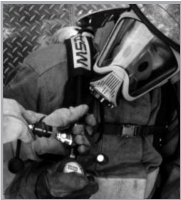
Near the fire scene, firefighters can quickly replenish their SCBA air supply without having to remove the air mask and with no need for cylinder change over.
