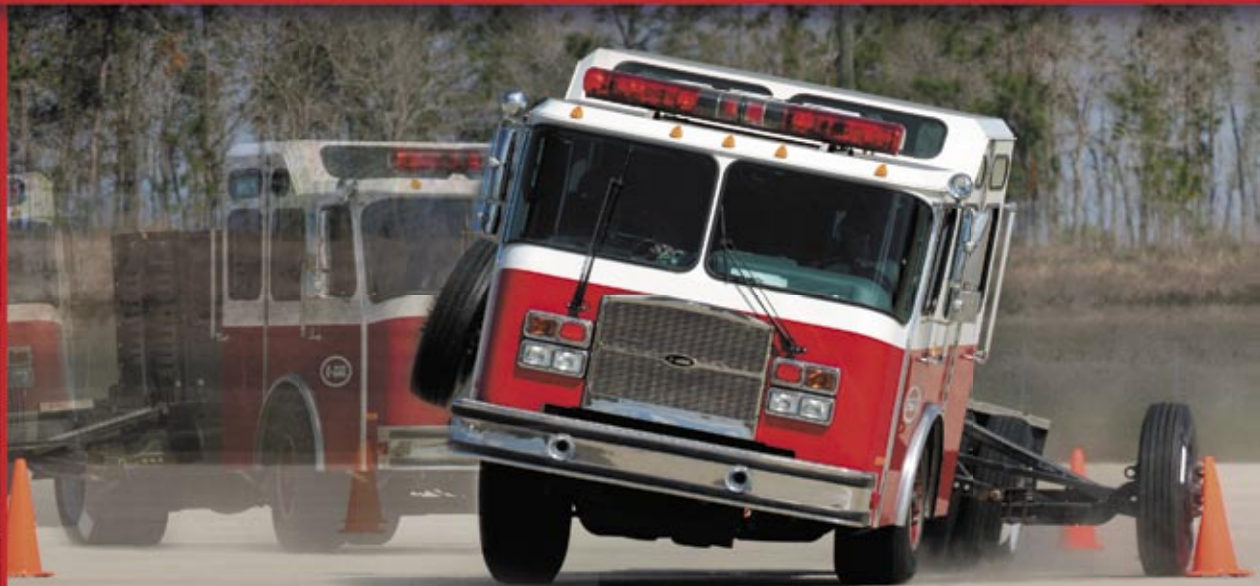
E-ONE CYCLONE TEST VEHICLE WITHOUT ROLL STABILIZATION.
