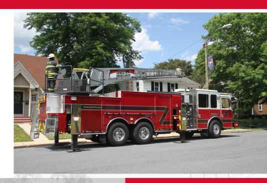
Designed with two sets of H style stabilizers fully extending to only 12' allows for positioning and unrivaled performance on an 11-degree slope.
